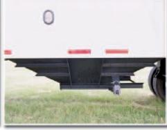
The hoppers on Maurer steel grain trailers are built to receive a retrofit side discharge chute. Anytime during the life of your trailer you can order a chute and add it to your trailer.
