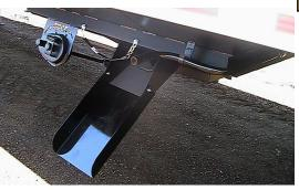
Side chute with extension shown. Chute extends 2" past side of trailer. Also shown is optional 2–speed gear reducer
