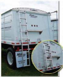
Demco Steel Grain trailers are equipped with LED sealed beam lights. Every light is mounted in a shock proof rubber grommet. Combine this with our wiring system and you can plan on years of trouble free use. Note the unitized corner which is an exclusive feature on Demco steel grain trailers
