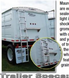
Maurer steel grain trailers are equipped with LED sealed beam lights. Every light is mounted in a shock proof rubber grommet. Combine this with our wiring system and you can plan on years of trouble free use. Note the unitized corner which is an exclusive feature on Maurer steel grain trailers.
