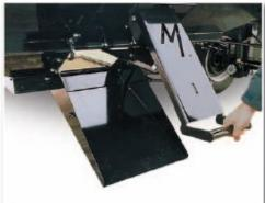
A Maurer side discharge chute has 9 inches of discharge height and 35° of slope while still reaching within 2" of the side of the trailer. These traits make this side discharge the most user-friendly on the market!
